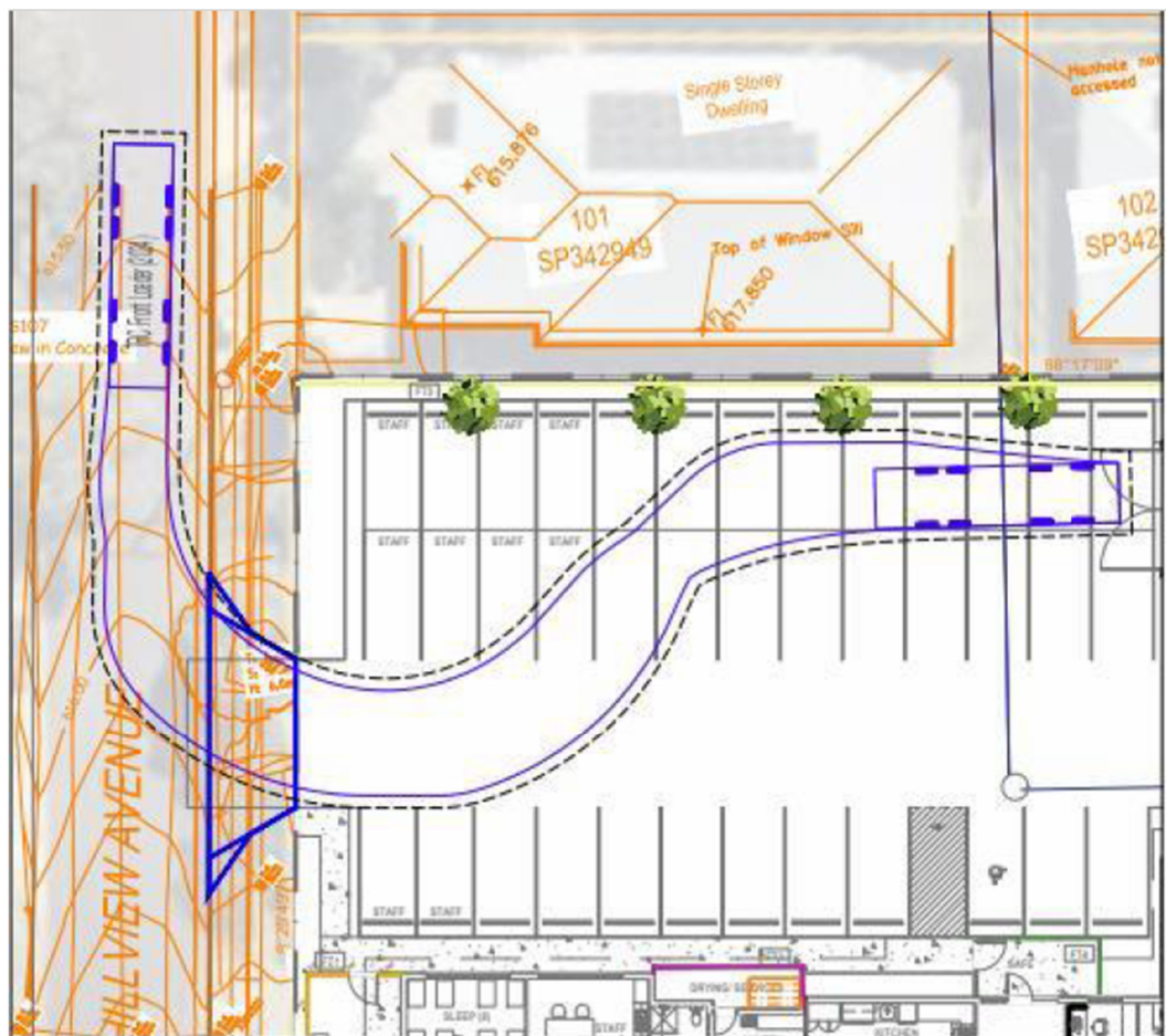
RCV - ENTRY MANOEUVRE
