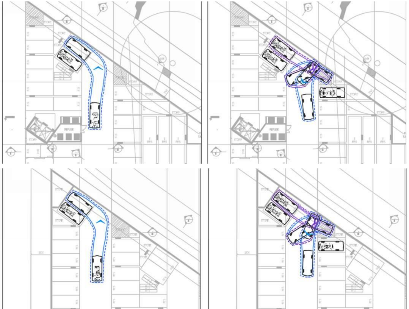
Figure 9 Basement - End bay - Swept Paths
