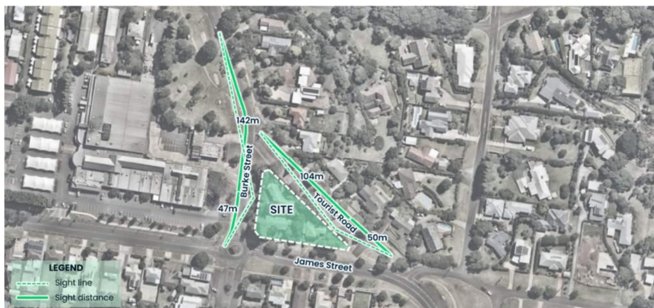
Figure 6 - Access sight distance
