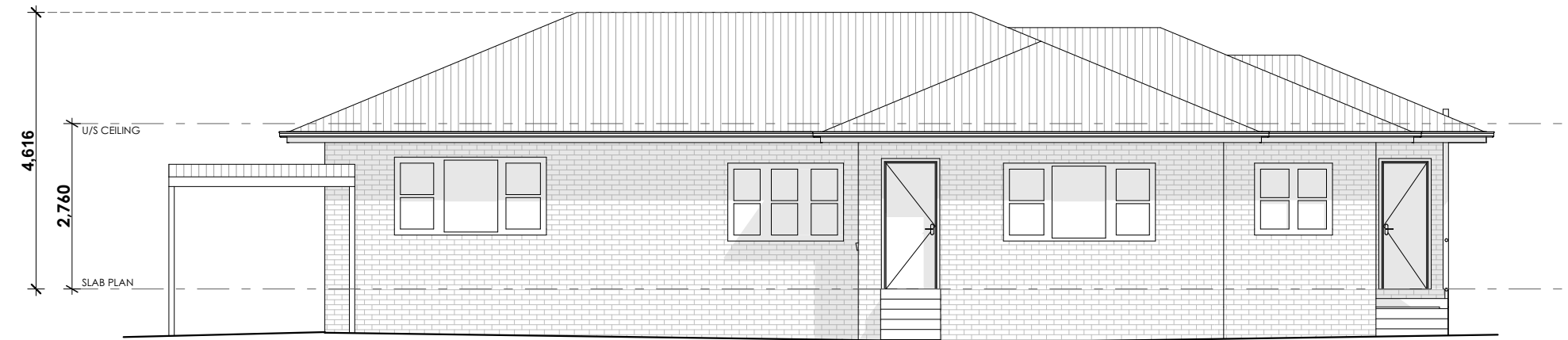
SOUTH ELEVATION - BUILDING B Scale: 1:100
