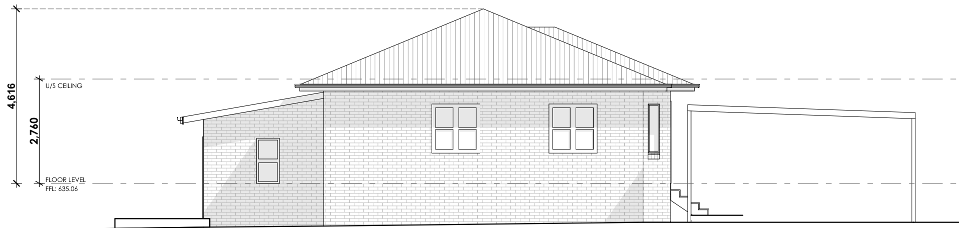
WEST ELEVATION - BUILDING B Scale: 1:100
