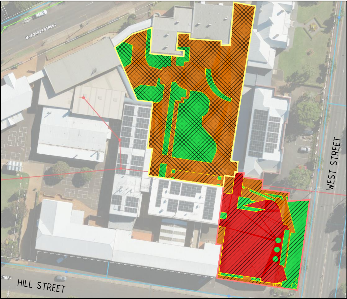
POST-DEVELOPED STORMWATER CATCHMENTS
