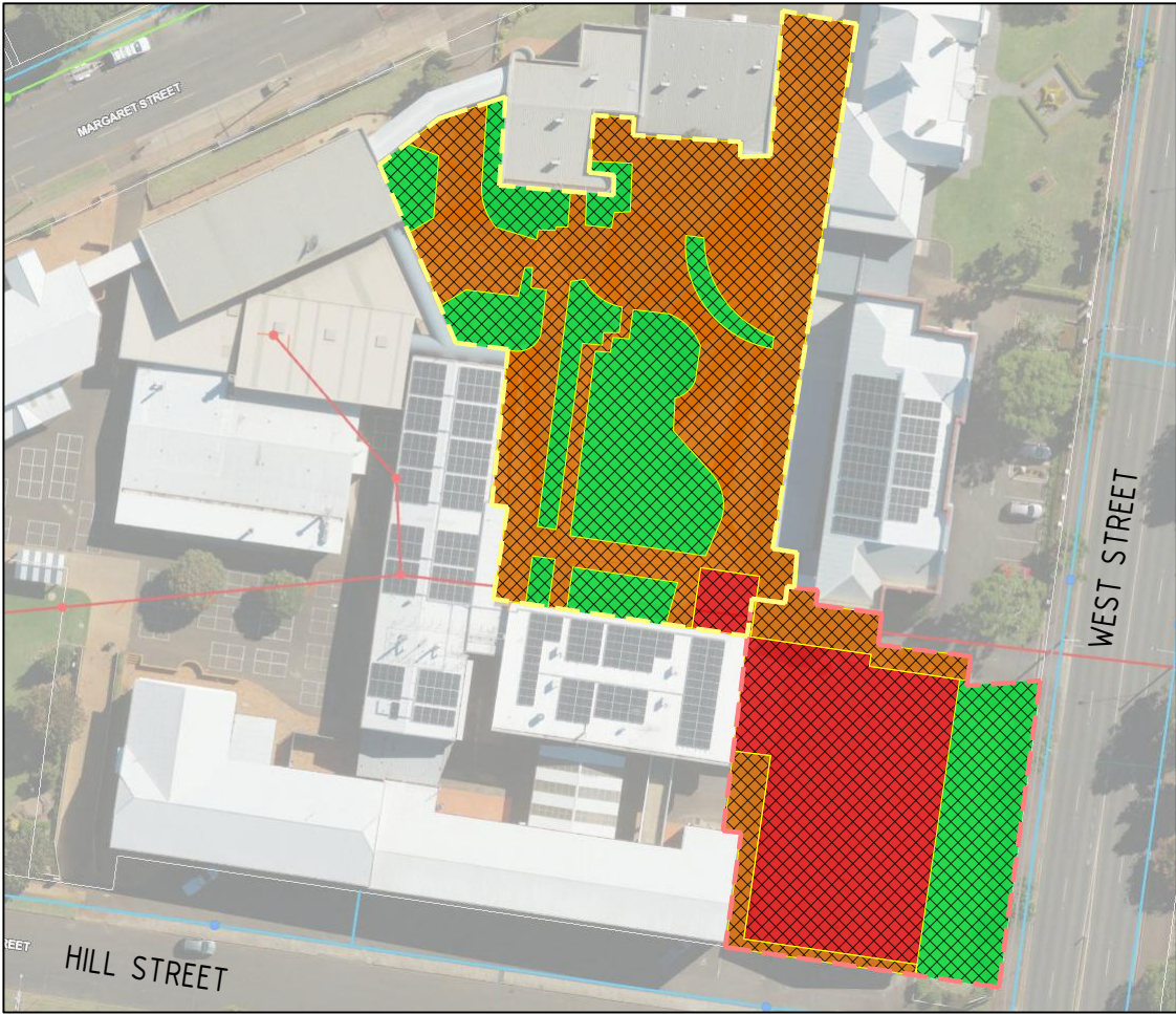
PRE-DEVELOPED STORMWATER CATCHMENTS
