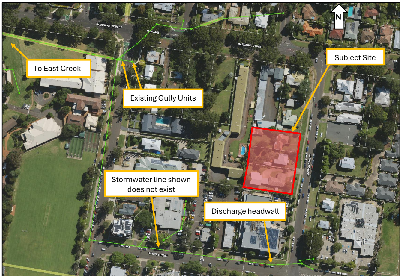
FIGURE 4 EXISTING STORMWATER NETWORK (TRC INFRASTRUCTURE MAPS 2026)
