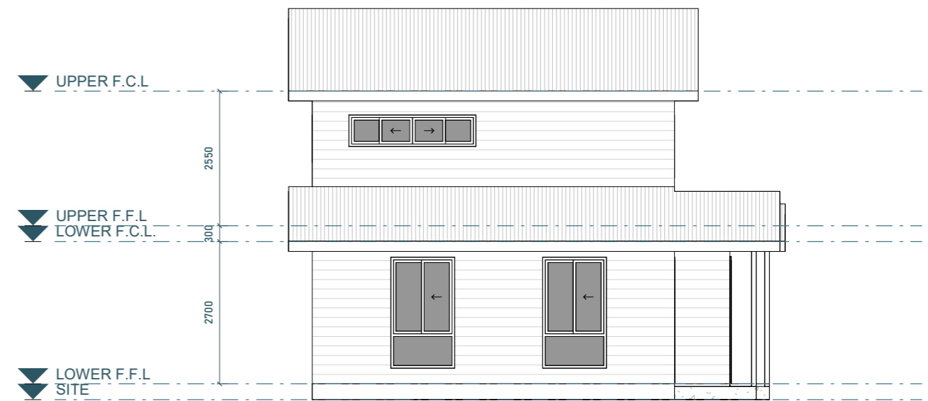
2 UNIT 6 - EASTERN ELEVATION 1:100
