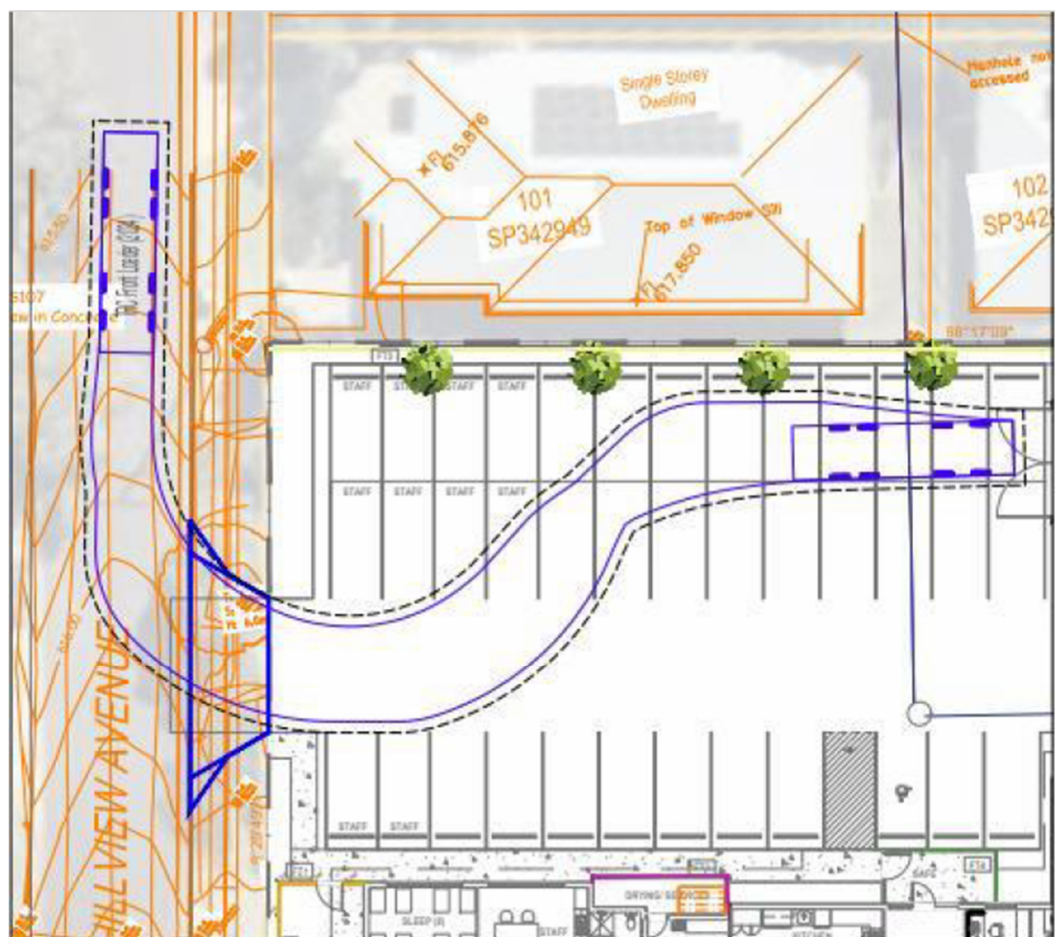
RCV - ENTRY MANOEUVRE
