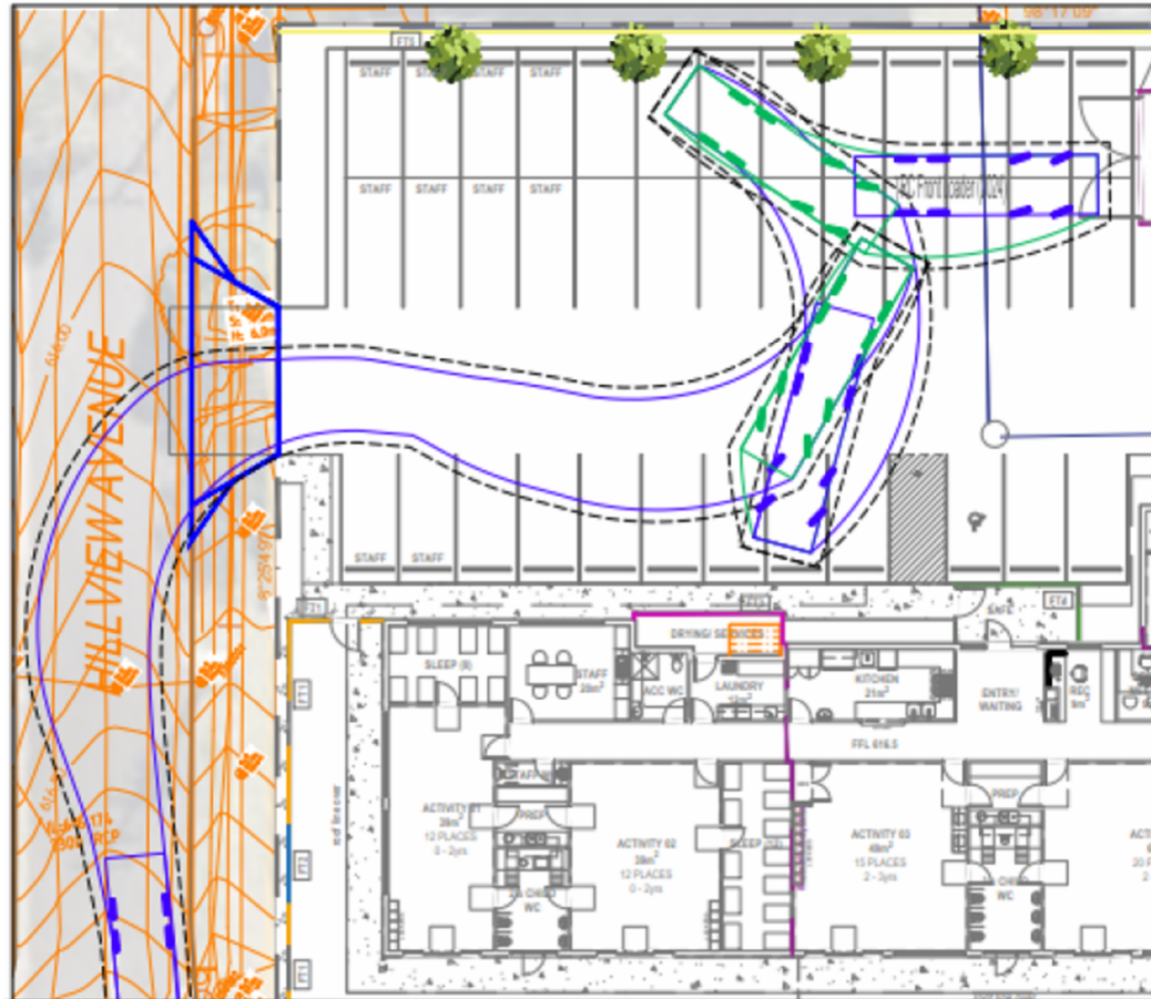
RCV - EXIT MANOEUVRE
