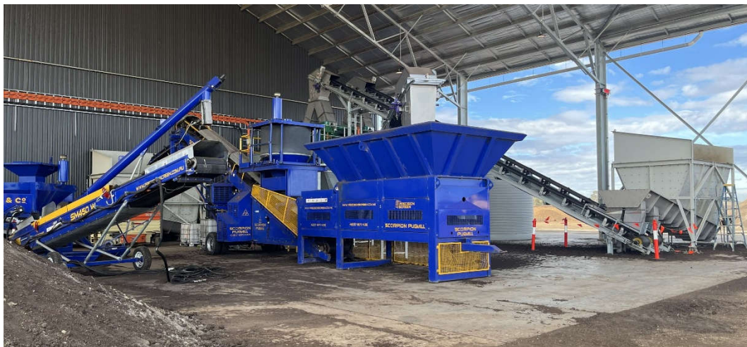
Fig 6 Blending and Pug Mill equipment
