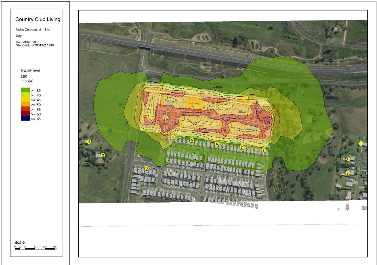
Noise contours at 1.8m for daytime cumulative variable noise sources. Levels are in dB(A), L_{eq,1hr}
