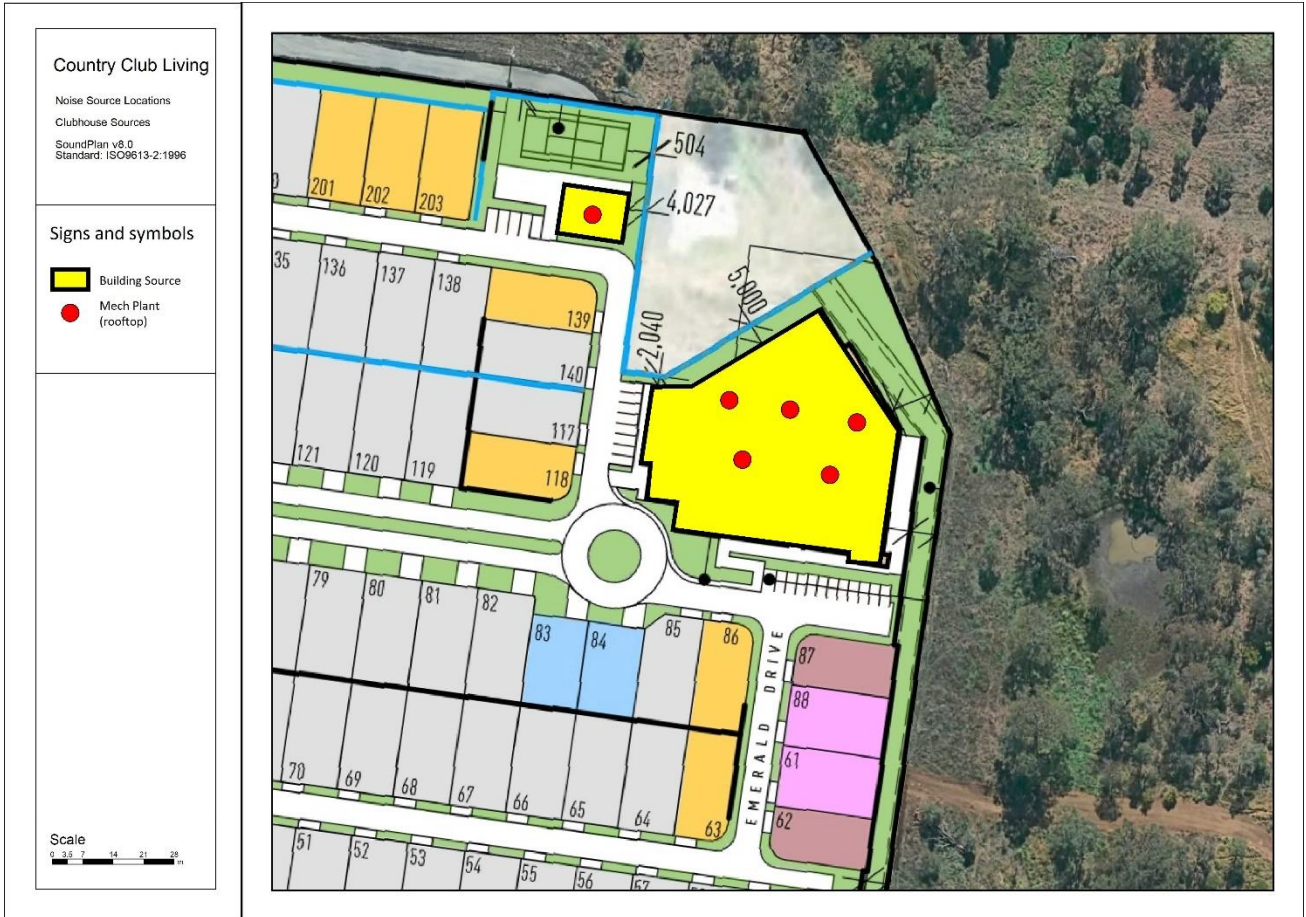
Clubhouse (including rooftop mechanical plant) noise source locations
