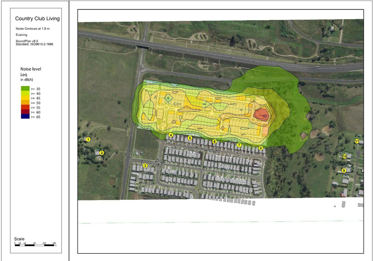
Noise contours at 1.8m for evening cumulative variable noise sources. Levels are in dB(A), L_{eq,1hr}
