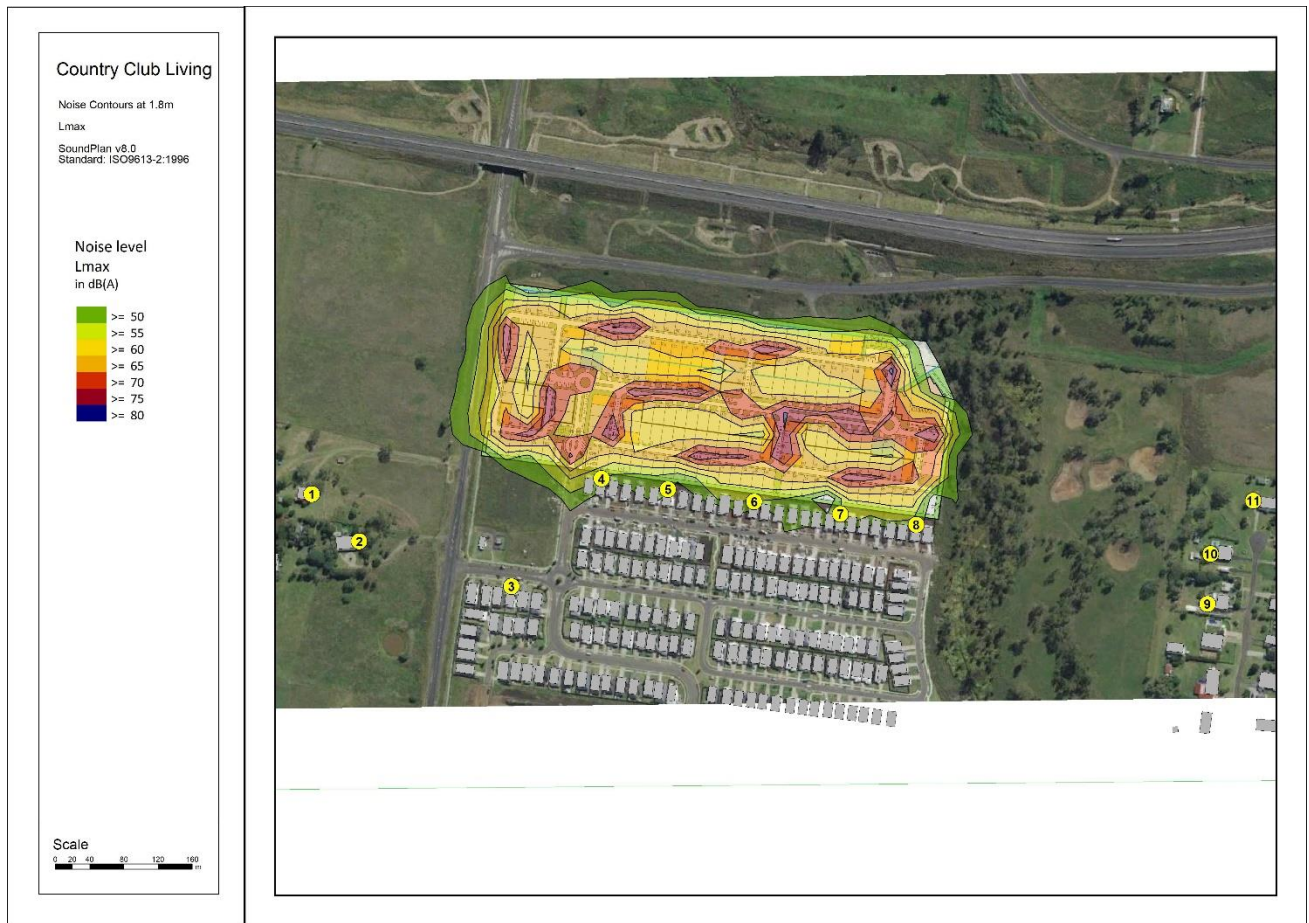
Noise contours at 1.8m for discrete noise sources during the night-time period. Levels are in dB(A), L max
