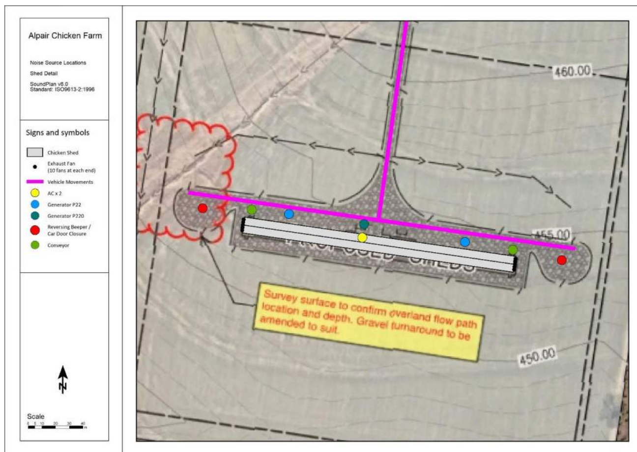
Figure 4 Detailed Shed Noise Source Locations
