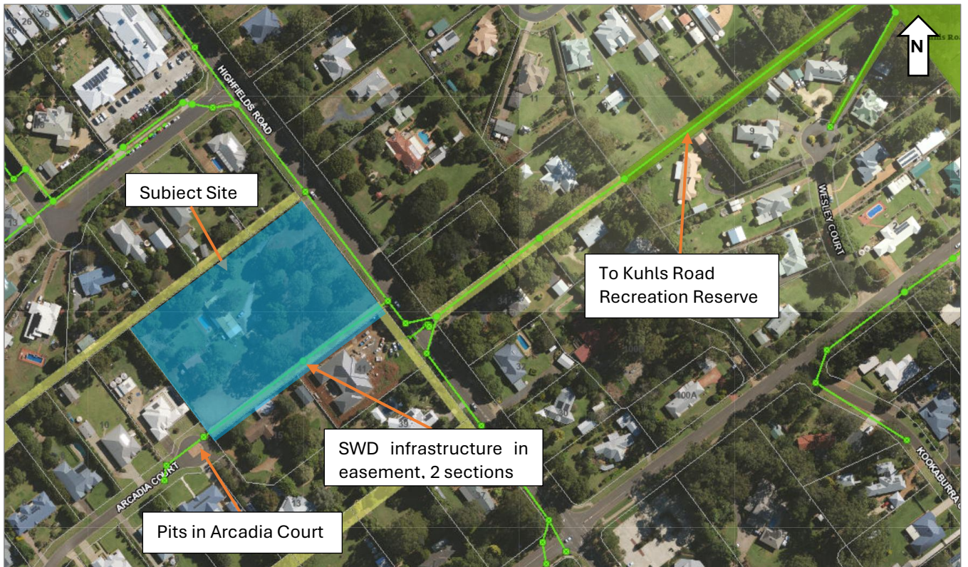
FIGURE 4 EXISTING STORMWATER NETWORK (TRC INFRASTRUCTURE MAPS 2026)
