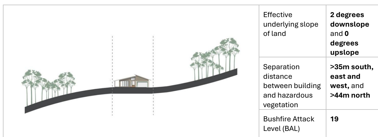
Figure 3 Determination of distance from classified vegetation and effective slope of land.
