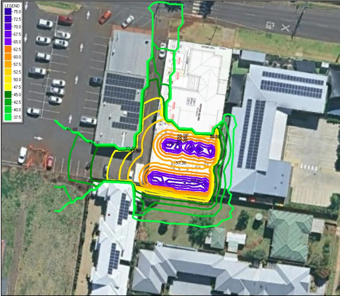
Plate B2: Noise contours at 1.8m, parking activity. Levels are in dB(A) L 01,1hr
