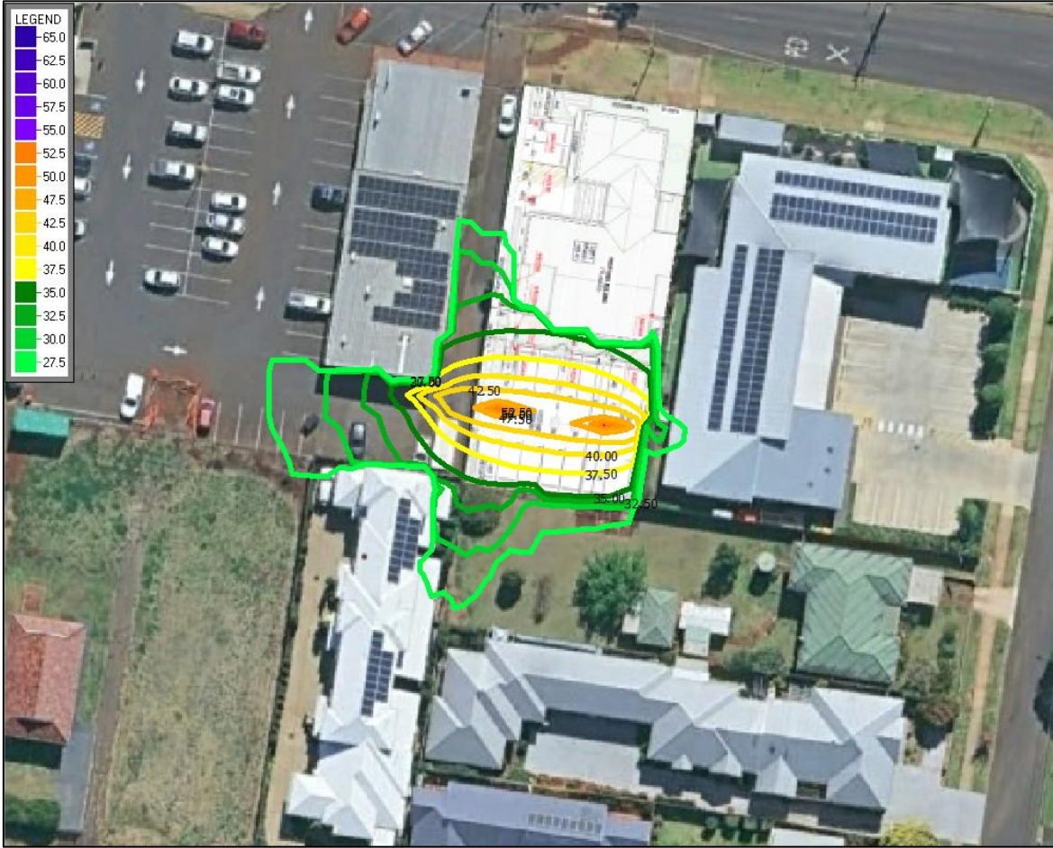
Plate B1: Noise contours at 1.8m, vehicle movements. Levels are in dB(A) L_{eq,1hr}
