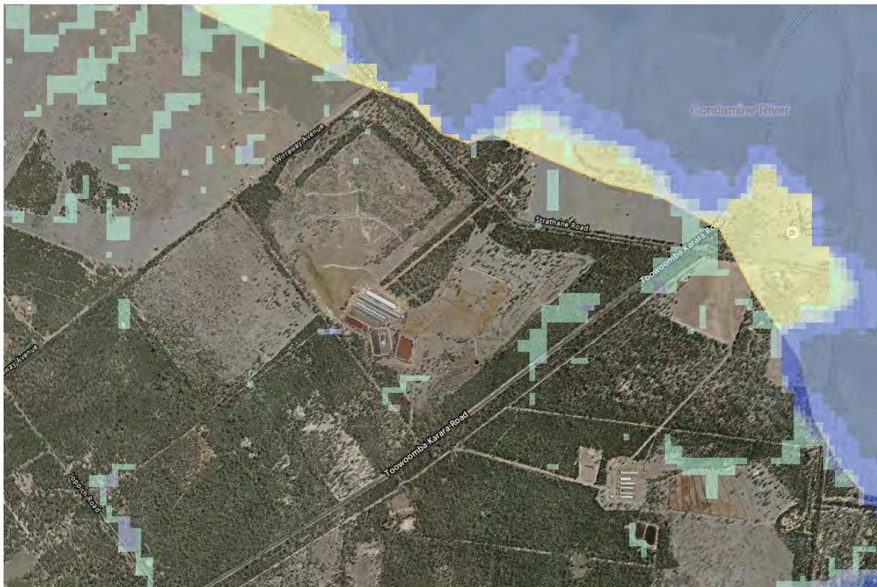
Figure 7 – Flood mapping – floodplain extent (yellow) and 1 % AEP mapping (blue). Source: FloodCheck Queensland
