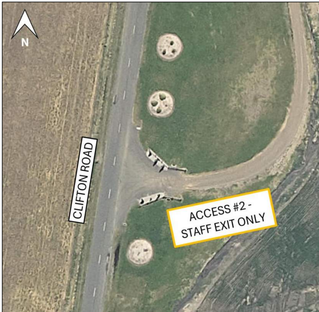
Figure 3-6: Clifton Road / Site Access #2 priority controlled T-intersection
