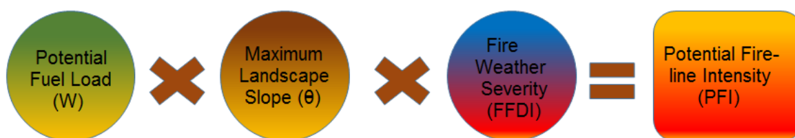
Figure 5: Variables used to determine Potential Fire-line Intensity. (Redrawn from Leonard et al 2013)
