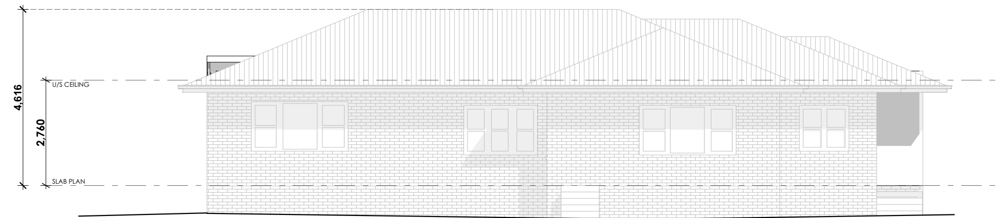
SOUTH ELEVATION - BUILDING B Scale: 1:100
