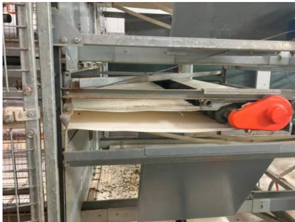
Photograph 4 – Manure belt and extraction
