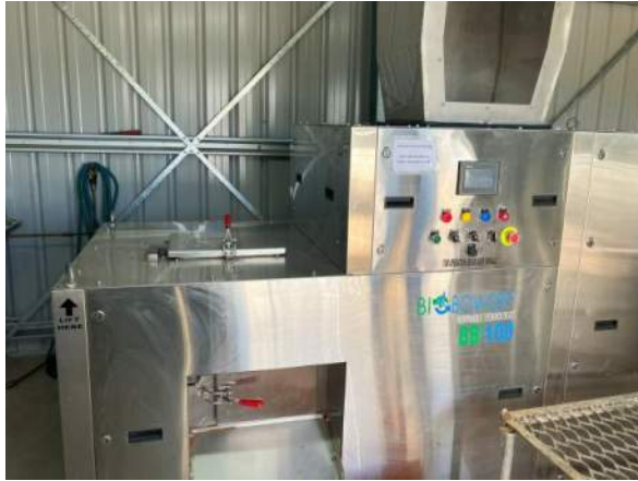
Photograph 3 – Biobowser accelerated composter
