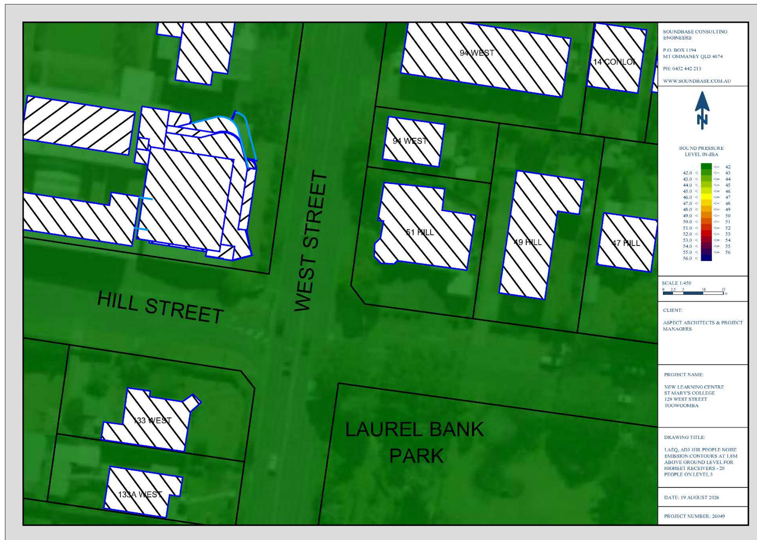
Figure 15: Highset L_{Aeq, adj, 1hr} noise emission contours for 20 people on Level 3
