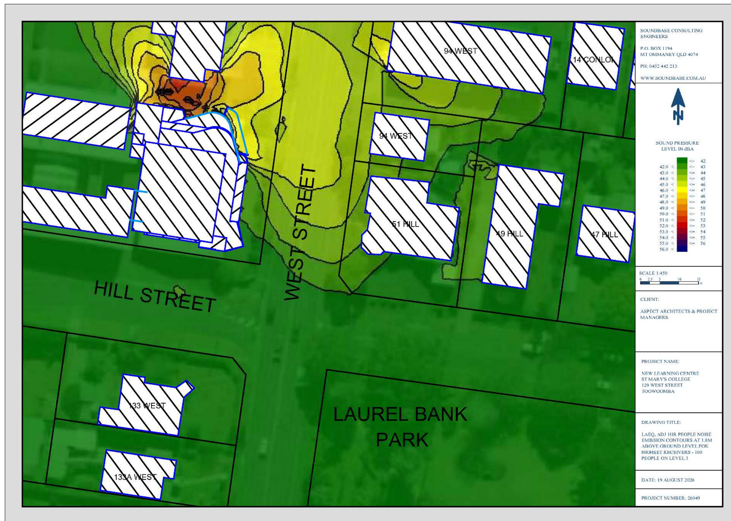
Figure 17: Highset L_{Aeq, adj, 1hr} noise emission contours for 100 people on Level 3
