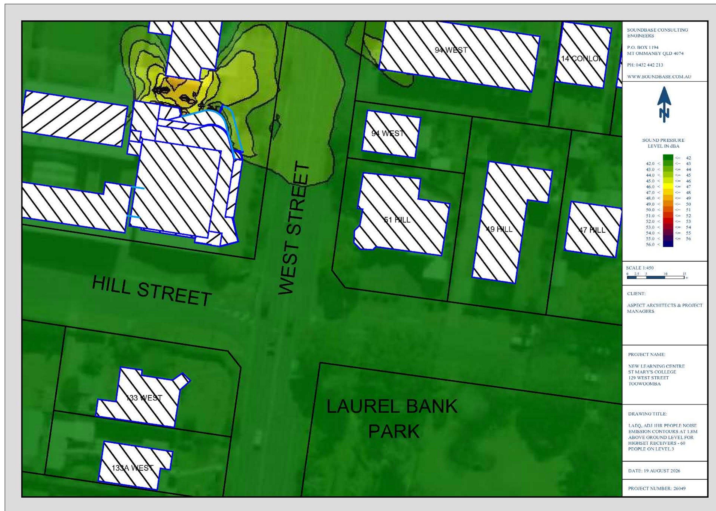
Figure 13: Highset L_{Aeq, adj, 1hr} noise emission contours for 60 people on Level 3
