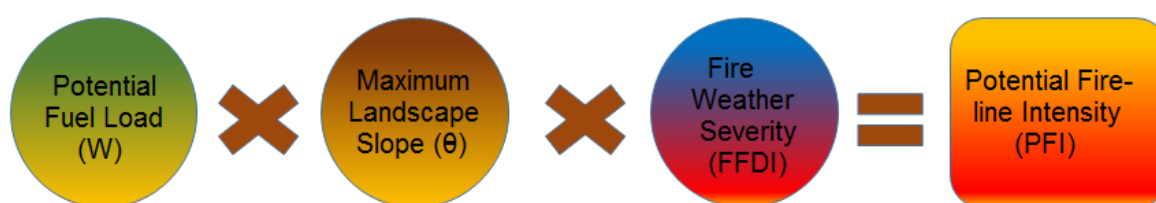
Figure 14 Variables used to determine Potential Fire-line Intensity. (Redrawn from Leonard et al 2013)
